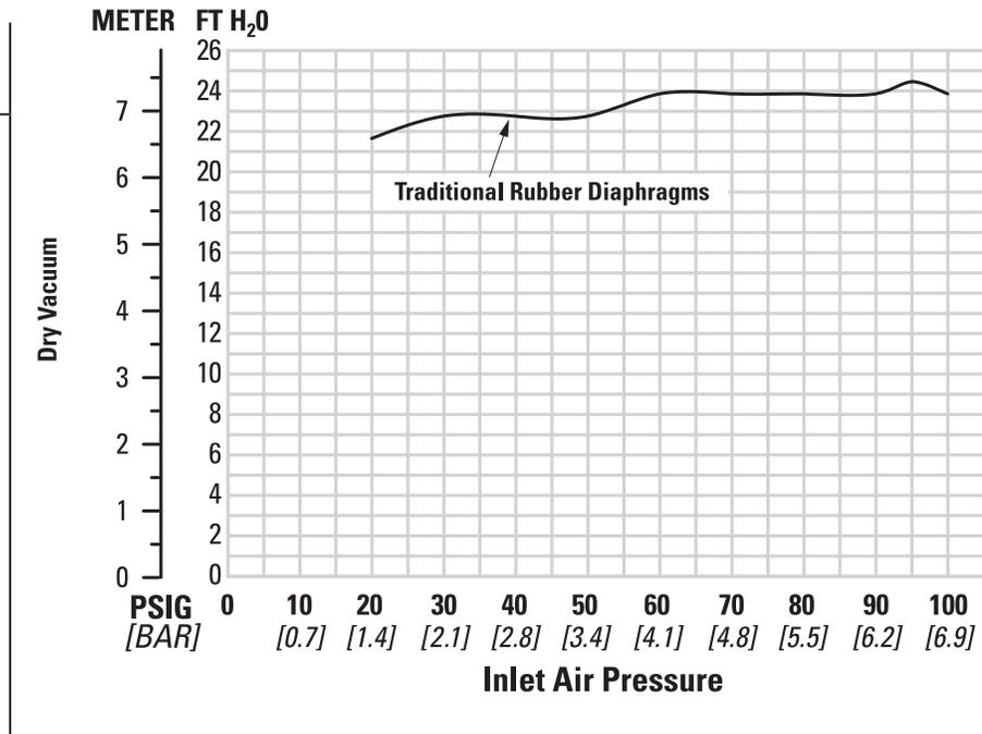
Suction-lift curves are calibrated for pumps operating at 305 m (1,000') above sea level. This chart is meant to be a guide only. There are many variables that can affect your pump's operating characteristics. The
