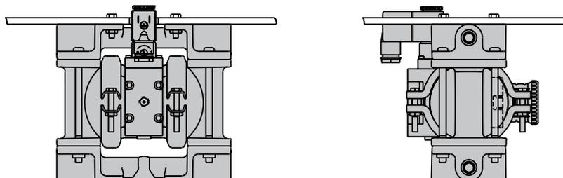
**CAUTION:** Pump performance will be seriously hampered if pump is installed upside down.
