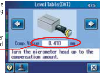
DAT screen guides the user when leveling Digimatic micrometer head Amount of micrometer head adjustment required Leveling table (DAT) (Option)
