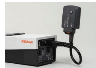
Example of the connection with SJ-210
