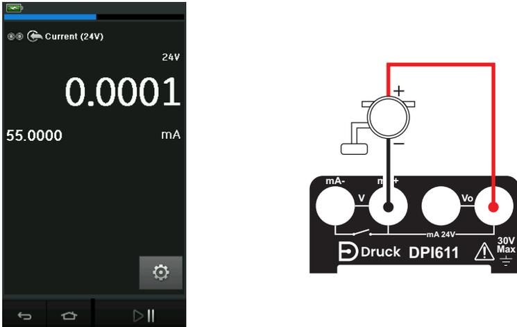
**Figure 2-17: Measure Current on CH1. Range  $\pm 55$  mA**
