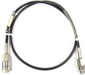
A high pressure pneumatic hose rated to 400 bar (5800 psi). The hose connects directly to the DPI611 pressure port and replicates the quick fit connection for compatibility with the standard adaptors supplied and the other adaptor kits.
