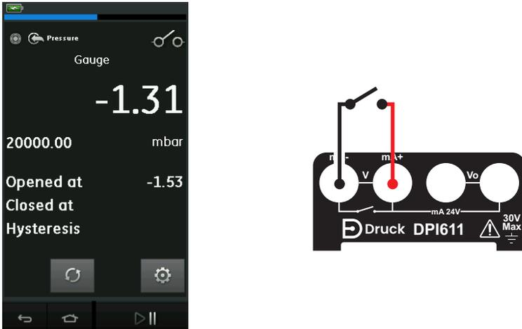
**Figure 2-21: Switch Test**
