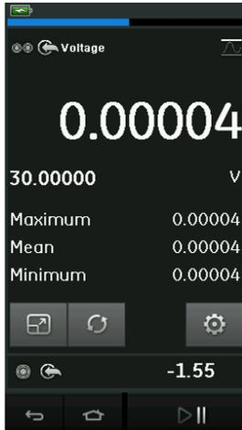
**Figure 2-11: Max/Min/Avg Example**
