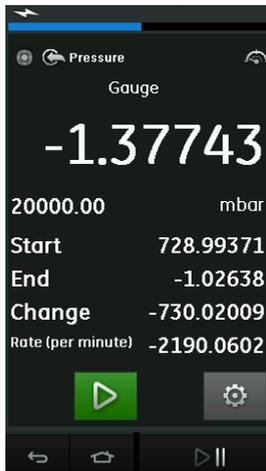
**Figure 2-24: Leak Test Example**
