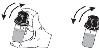
In order to avoid reagent leaking and to obtain more accurate measurements, close the cuvette first with the supplied HDPE plastic stopper
