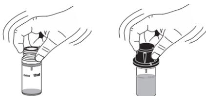
In order to avoid reagent leaking and to obtain more accurate measurements, close the cuvette first with the supplied HDPE plastic stopper
