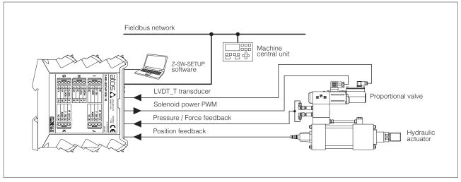
Note: block diagram example for alternated position/force control, with fieldbus interface
