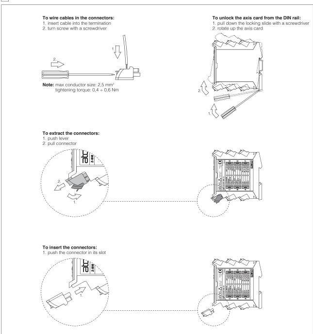
Note: all connectors are supplied with a mechanical coding. This feature ensures a unique insertion of each connector in the own slot. (eg. connector A can not be inserted into connector slot of B,C,D,E,F,G,H,I,J,K)
