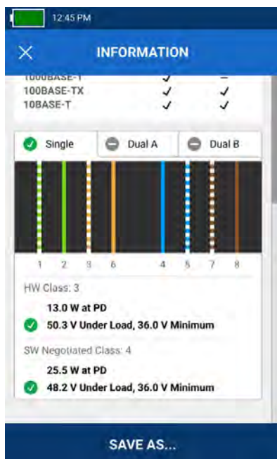
Switch port Power over Ethernet result shows pairs used, power and class available and results of the PoE test under load.
