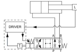
one load cell transducer has to be installed between the actuator and the controlled load. The SL option directly control the actuator force
