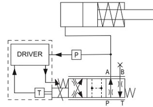
one remote pressure transducer has to be installed on the actuator's port to be controlled. In this example the SP option regulates the pressure on port A
