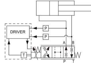
two remote pressure transducers have to be installed on the actuator's ports A and B. The bore and rod dimensions of the actuator have to be input into the valve software, which calculates the relevant areas: A1 = bore area; A2 = ring area. The SF option directly controls the actuator force (F) as result of the following calculation:  $F = (P_a \times A_1) - (P_b \times A_2)$
