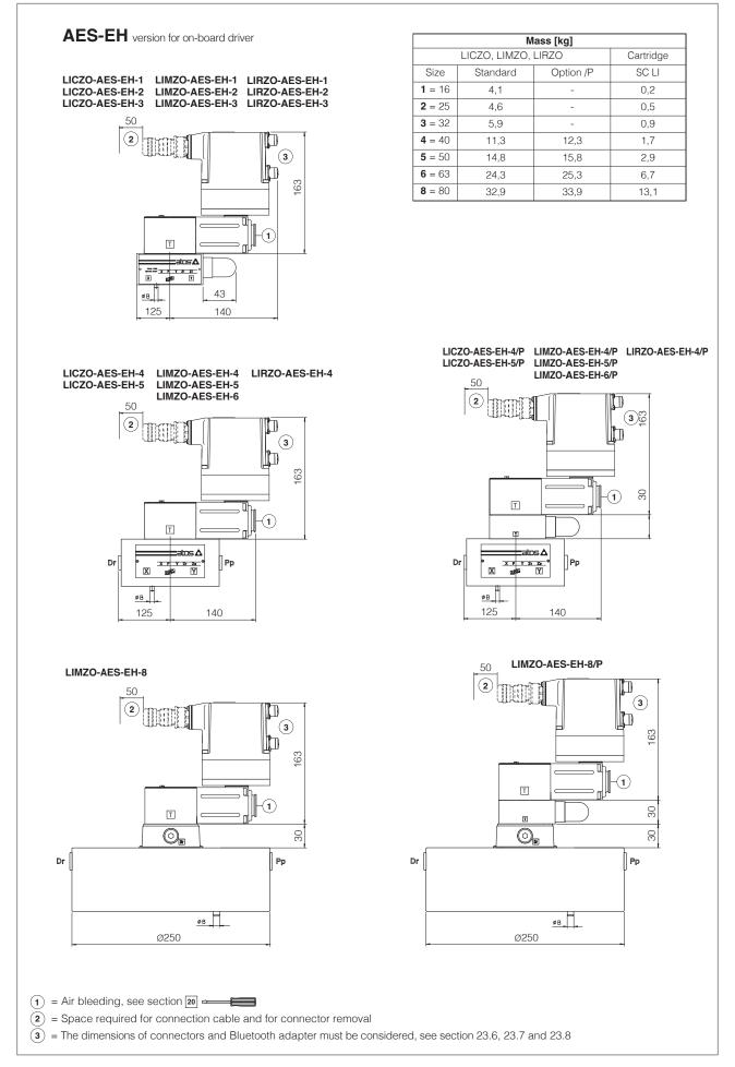
Note: for mounting surface and cavity dimensions, see tech. table P006
