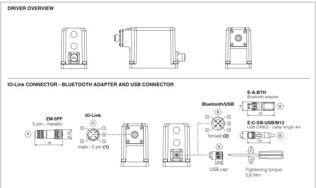
(1) Use of metallic connectors is strongly recommended in order to fulfill EMC requirements (2) Pin layout always referred to driver's view
