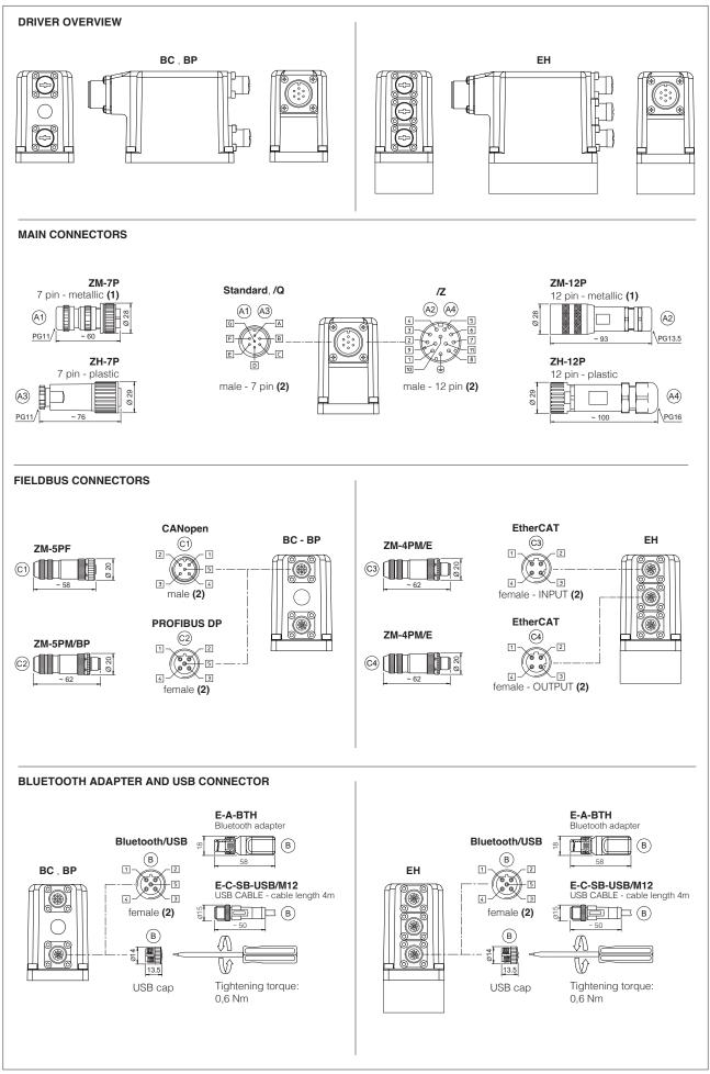
(1) Use of metallic connectors is strongly recommended in order to fulfill EMC requirements (2) Pin layout always referred to driver's view
