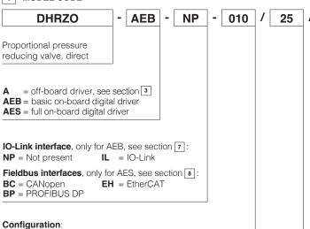
010 = reduced pressure on port A 012 = reduced pressure on port A and B
