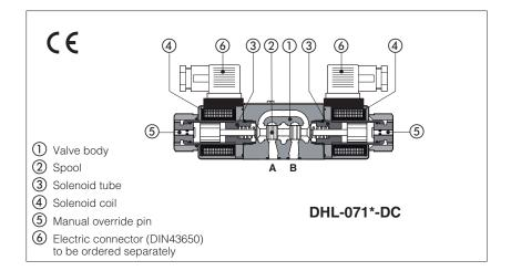
Spool type, 4/3, 4/2, 3/2 way version. Wet type solenoids made by:
