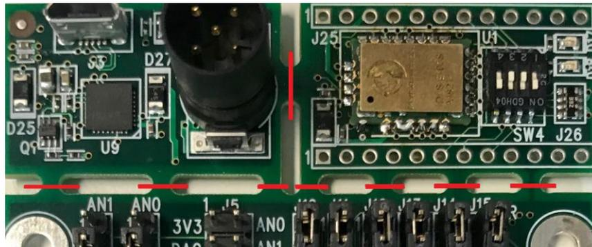
**Figure 3.6.** cut the board on the following lines
