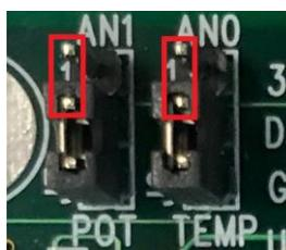
**Figure 3.3.** Auxiliary external analog inputs selected J6..J7
