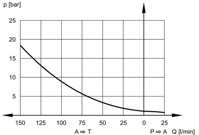
Pressure drops A → T as a function of the flow rate, without any backpressure in T and with command signal = 0V
