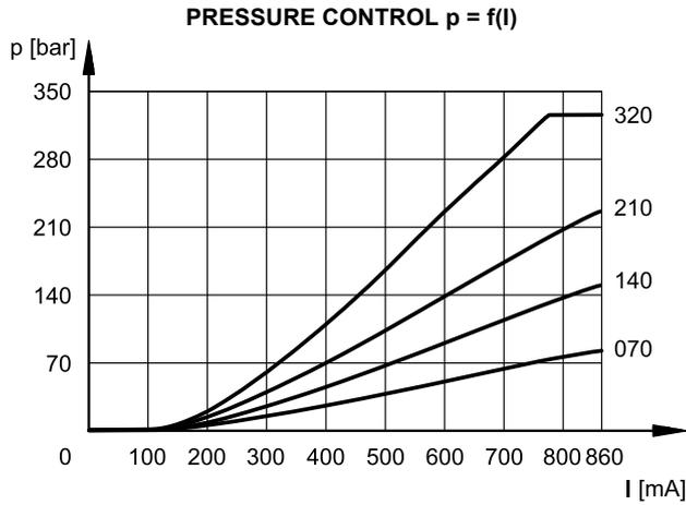
Characteristic curves as a function of the current to the solenoid for the available pressure adjustment ranges, obtained with A port plugged.
