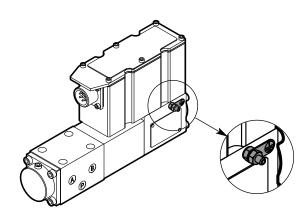
The grounding point must always be wired with the general earthing system by means of a suitable conductive line.
