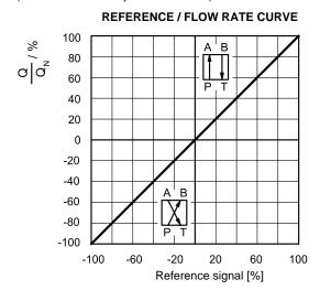
Typical flow rate curves at constant  $\Delta p = 70$  bar P-T according to the reference signal.
