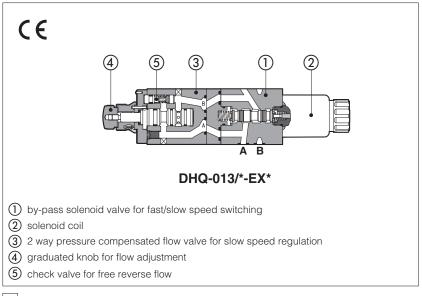
**DHQ** are modular valves for fast/slow speed control of hydraulic actuators.
