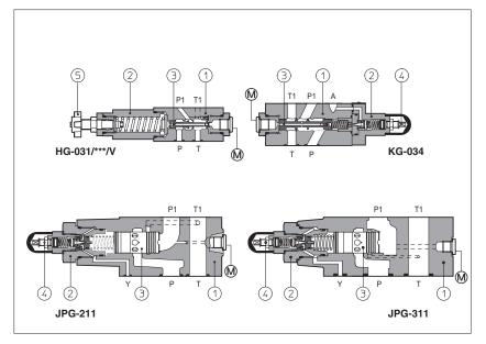
HG, KG, JPG are pressure reducing valves, spool type (3), designed to operate in oil hydraulic systems.
