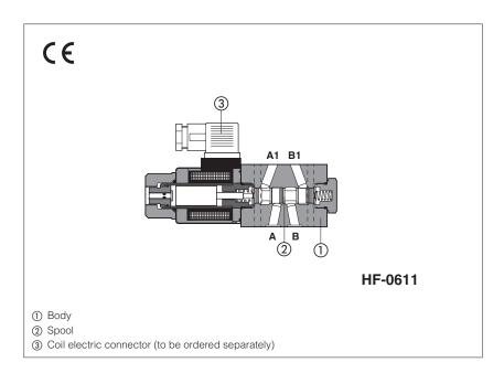
**HF** are spool type, direct operated solenoid valves in modular execution, normally used for shut-off or to by-pass the hydraulic user lines.
