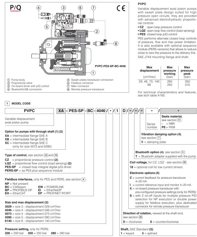
(1) For the LQZ and PERS versions, it must be checked that the pump to be coupled does not mechanically interfere with manifold and the OUT port of the first pump - consult our technical office
