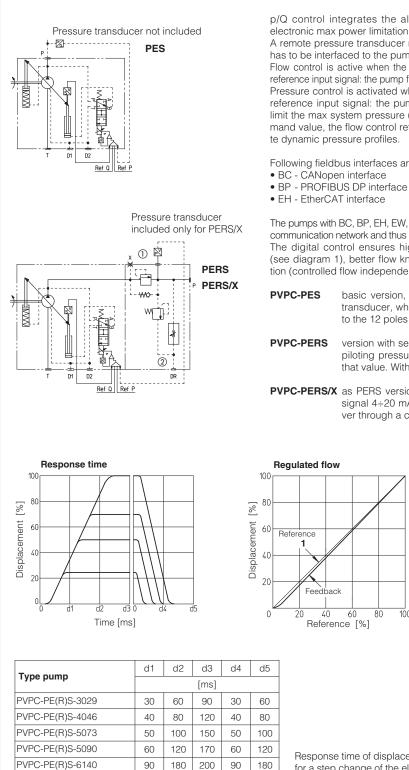
p/Q control integrates the alternate pressure and flow regulation with the electronic max power limitation. A remote pressure transducer must be installed on the system and its feedback
