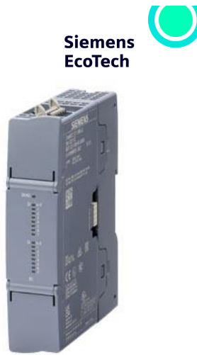
SIMATIC S7-1200 G2: SM 1231 analog input, 8 AI; inputs: 8x AI 14 bit ADC (+/-10 V, +/-5 V, +/-2.5 V or 0-20 mA/4-20 mA)
