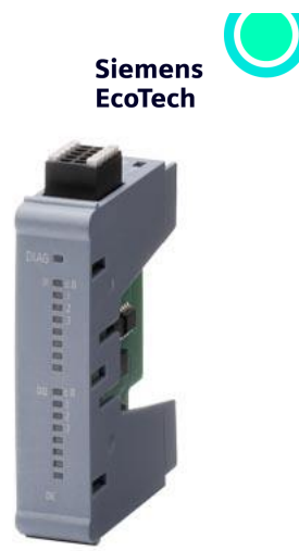
SIMATIC S7-1200 G2: SB 1231 analog input, 4 AI; inputs: 4 x AI 14 bit ADC (+/-10 V, +/-5 V, +/-2.5 V or 0-20 mA/4-20 mA)
