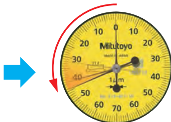
Indicator trackability depends on maintaining gear-train stability
