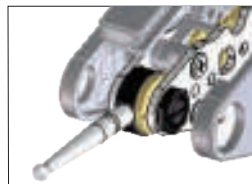
Stylus bearing screw held in sub-plate.
