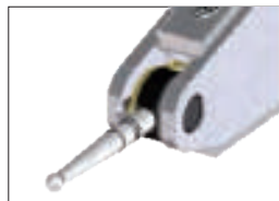
Stylus bearing screw held in frame.
