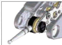
Stylus bearing screw held in sub-plate.
