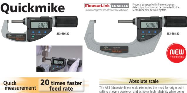
The Quickmike provides a speedy spindle feed of 10 mm per thimble rotation that enables widely differently sized features to be measured guickly. Also, 1-2"/30 mm of wide measuring range, which is .2"/5 mm longer than the standard type, allows measurement of multiple workpieces.
