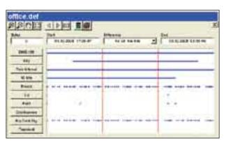
Overview of data for each measurement function. The user can save data transfer time by selecting which data is to be downloaded to the PC.
